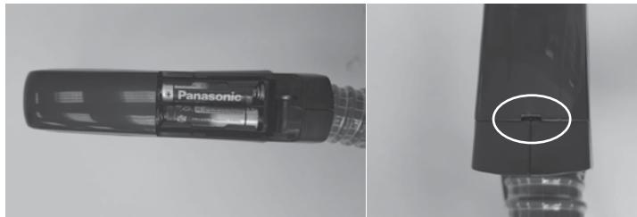
After installing / replacing the batteries, push battery compartment forwards to lock into its location.
