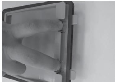
Pull the filter from the plastic set and shake it off to clean.
