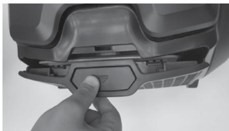
ESF, Pollen and H.E.P.A 13 / Active Carbon Filter cartridge shall be removed by pulling from the notch on the right.
